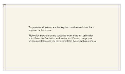
Step 7 After the calibration is complete, the Digitizer Calibration Tool dialog box will be displayed. Click Yes to save calibration data.
